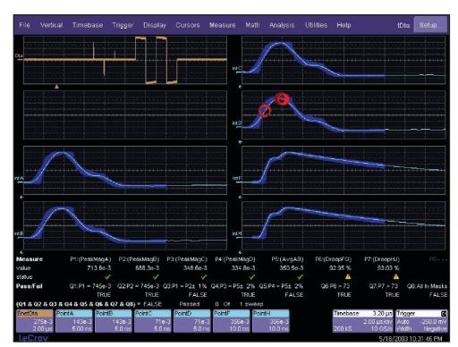
All mode 1 Gigabit Ethernet masks can be performed on one acquisition and displayed along with the voltage levels and droop.
